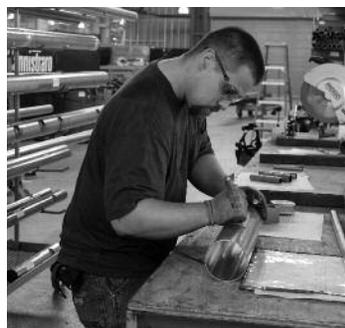
The FID includes a computer-controlled automatic pipe cutter, but employees such as Brian Janiak deburr pipes by hand.
